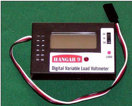
**A common mistake is to use a straight voltmeter to check voltage without a load to test a battery.** This is a waste of time as explained below. Lipos use a slightly different tester that checks individual cell voltage and resistance.
