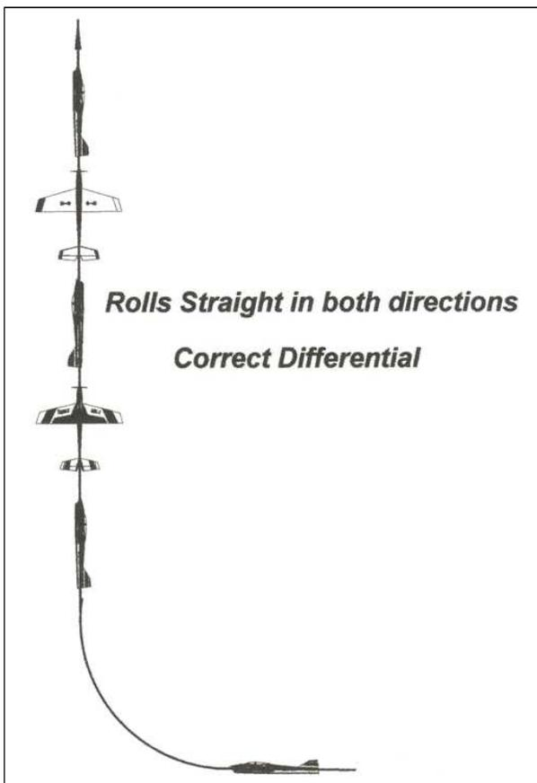
**Plane rolls on its longitudinal axis when differential is properly set**
