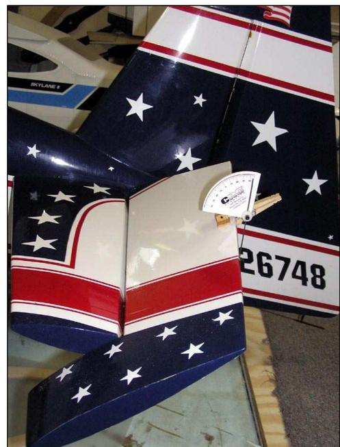
*This photo shows the 3D travel being checked and set with a throw meter set to 44 degrees which on my plane is plenty for 3D maneuvers as I fly with expo and the CG set on the rear limit.*
