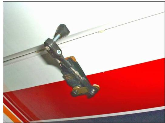
*Look close at this photo or enlarge it. Shown is a 1¼" servo arm with the ball link in the second hole position and the control horn fitting screwed all the way out. The distance from the hinge line to the pivot point on this plane is about 1¾" keeping the ratio on the safe side of the 1:1 ratio discussed earlier.*
