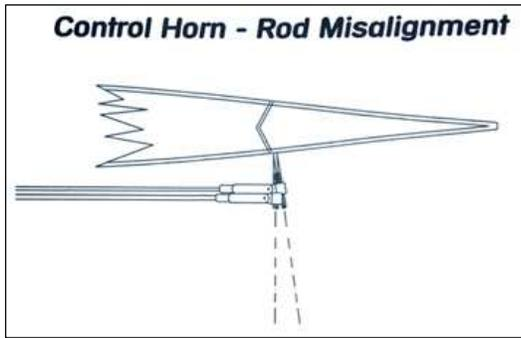
The misalignment on these threaded control horns on the right elevator or aileron compared to the left side will cause unequal travel relative to each other. Fix this control horn misalignment before going further. Additionally, if your linkage is 30 turns out from the hinge line on a threaded control horn, to the clevis on 1 side, and 33 turns out on the other side you will experience unequal travel making it impossible to properly trim the plane.
