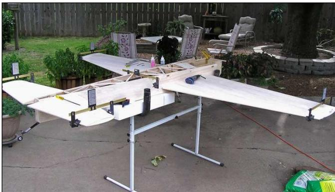
Shown is my 40% Carden Extra 300. Incidence meters are used to check wing and stab alignment relative to the longitudinal axis of the aircraft. The photo above shows 4 meters being used. One on each tip of the stab and wing. You can use one meter if that's all you have, it just takes longer. (Robart incidence meters work great).
