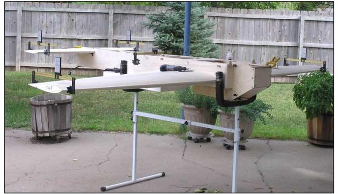
If you look close you can see the T Pin stuck in the top center of the firewall by the clamp that is "Home Base" for trammeling the aircraft with a piece of sewing thread.
